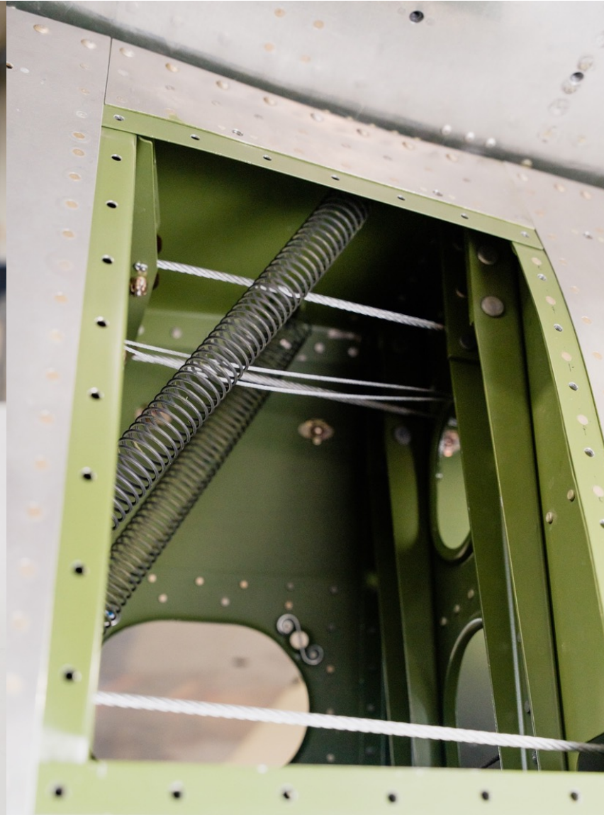
The large upper cable is an elevator control cable. Below that, the smaller cables are rudder trim cables. Finally, the large cable near the bottom of the opening is the rudder cable.
