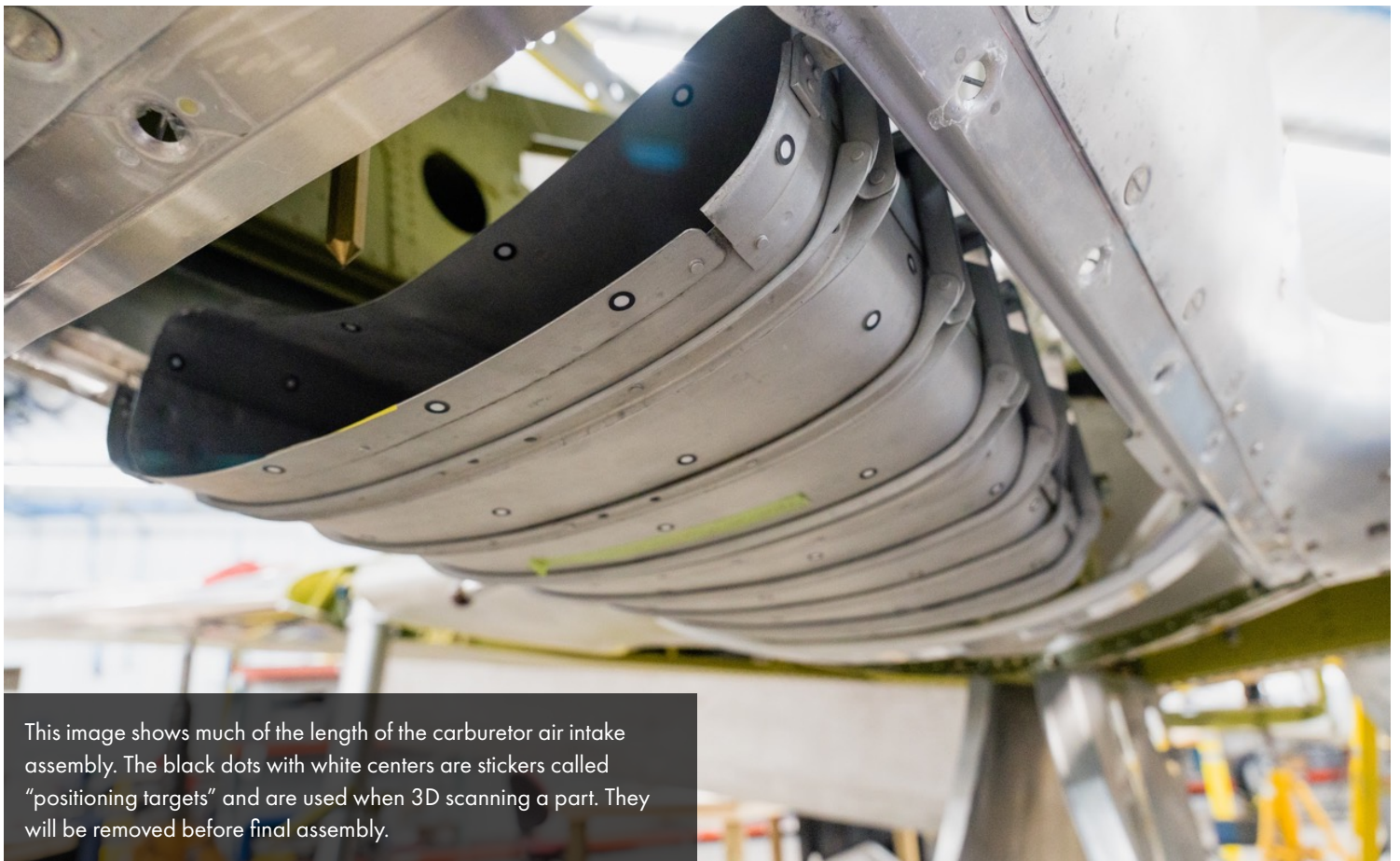
Mike works on the fit of the carburetor air intake duct assembly.
