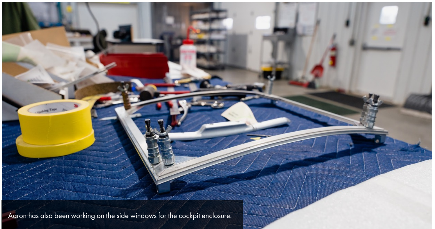
Tape protects the window from scratches as the part is checked for final fit.
