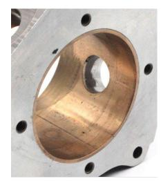
Note that the above assemblies had been refurbished from the factory or in the field. This was an original parker valve that was repaired but leaked due to scoring.
