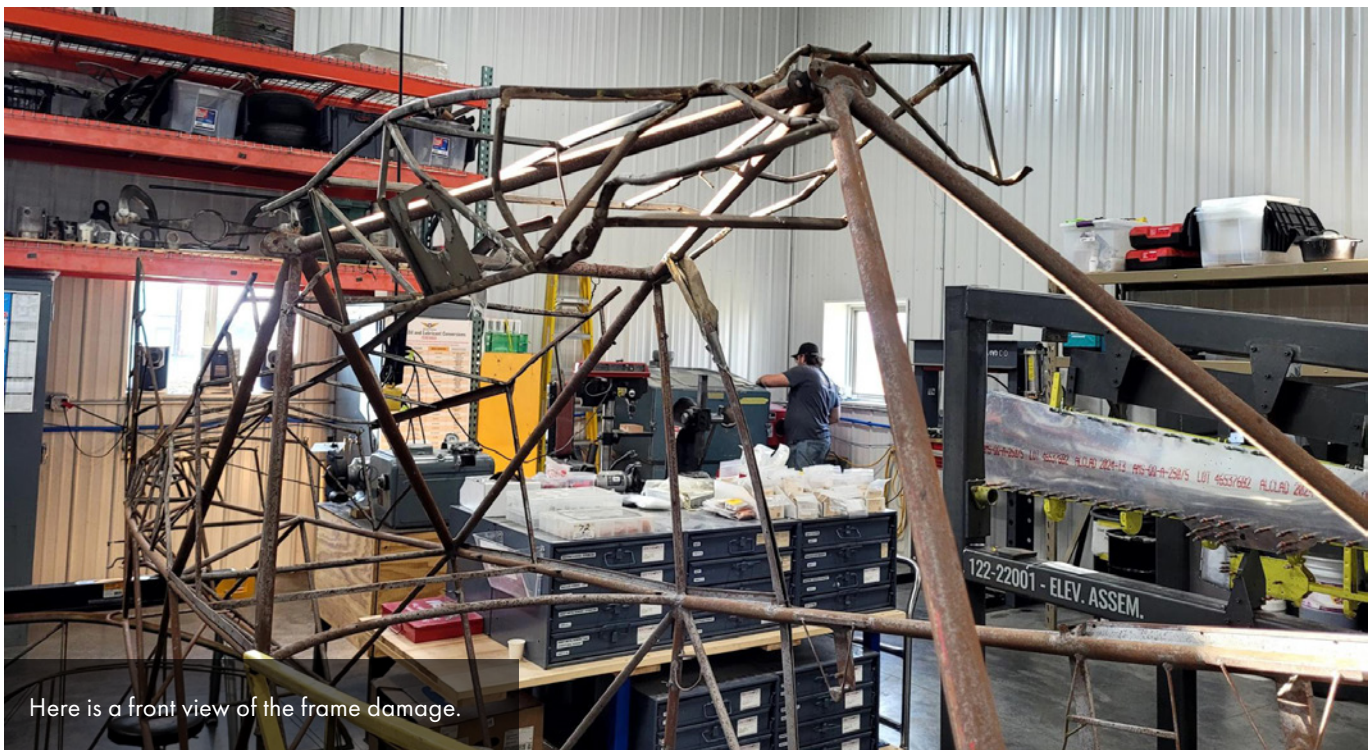
Fuselage frame damage corresponds to the crash damage evident in the accident photo.
