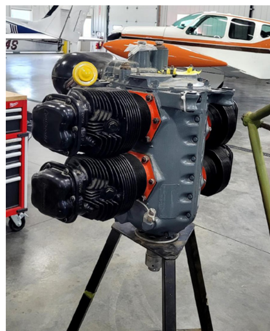
The nicely painted crankcase from the A-65 engine that came with the project.
