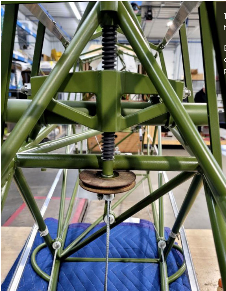
The cables from the jackscrew run forward to the trim control.
