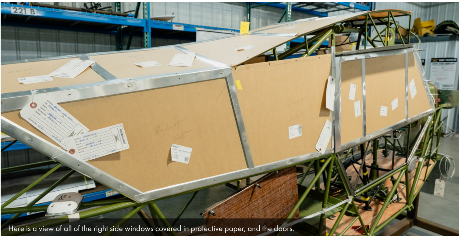
The rear right side window is one of the attributes that is different on an L-4 from a standard J-3
