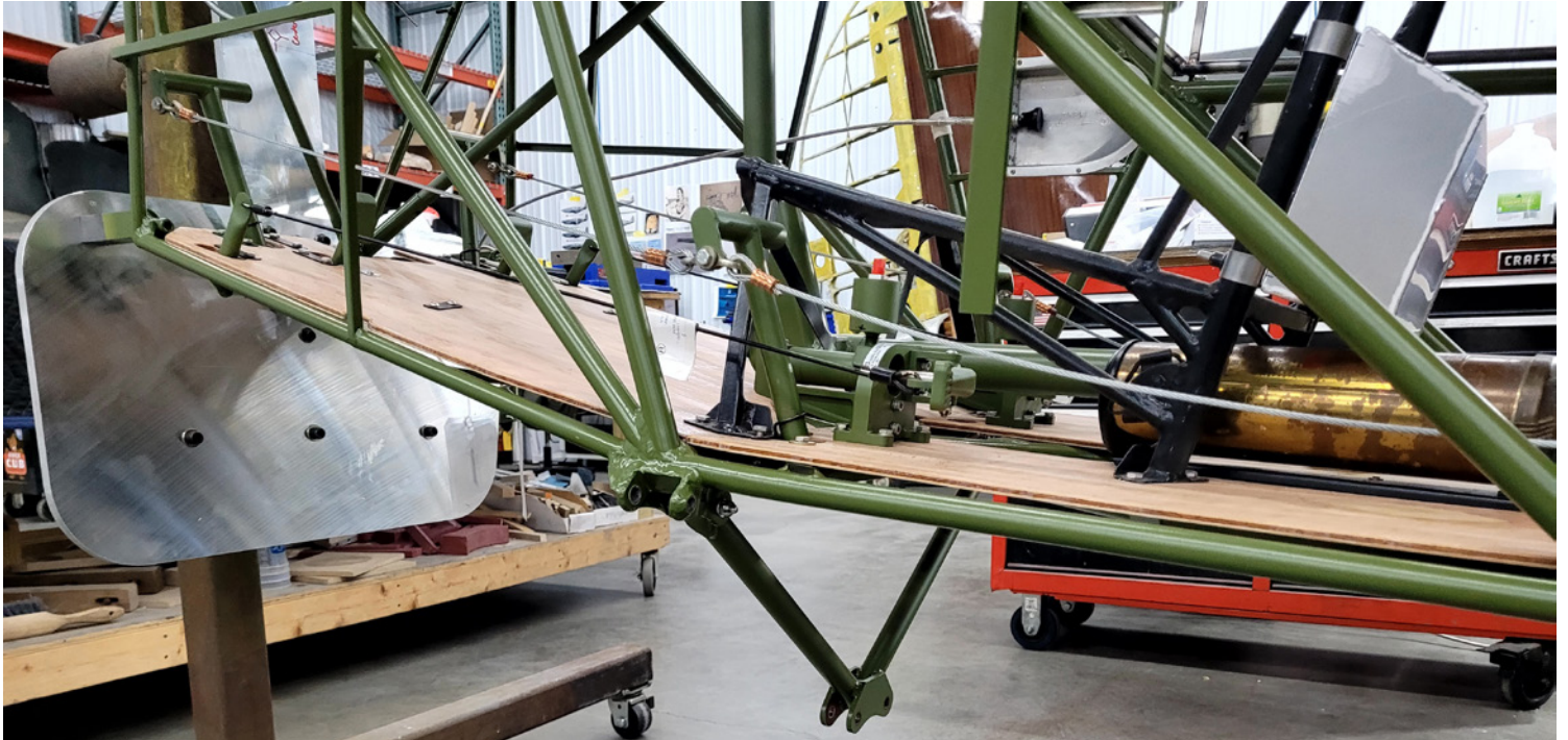
Returning to the L-4, the landing gear cabane vee was mounted before the main gear legs could be installed.
