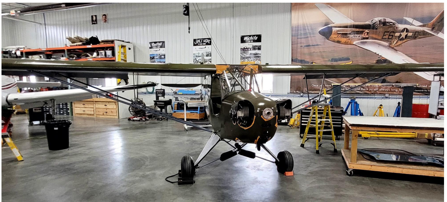
The L-4H has all the wing struts in place. The next step will be the wing root fairings that bridge the gap between the fuselage and the upper surface of the wings.
