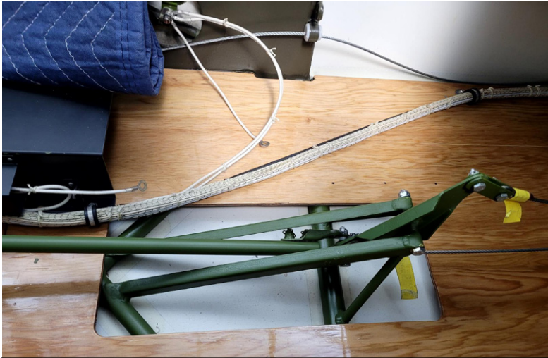
The tubular push rod from the two control sticks connects to a bellcrank that is linked to the elevator by cables.
