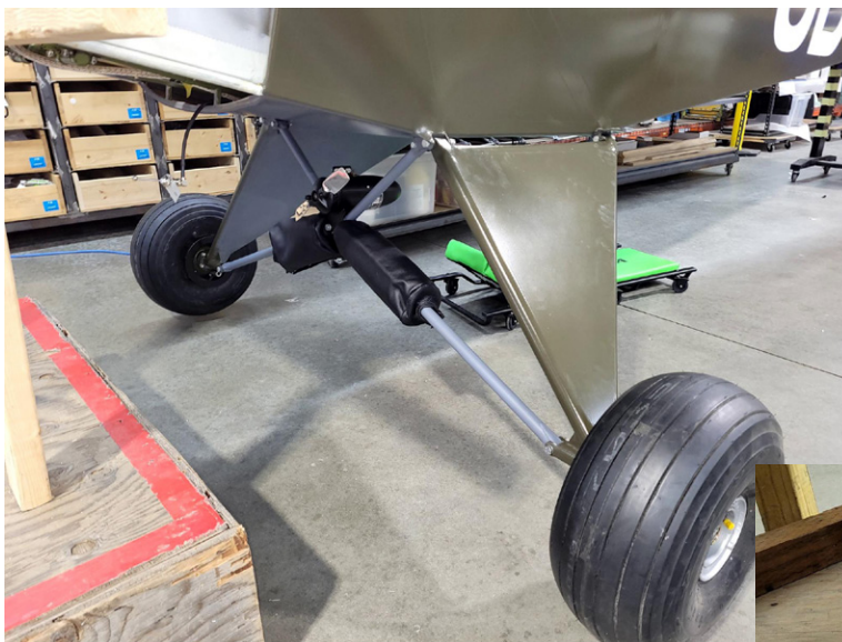
The landing gear bungee covers are one of the identifiers that you are looking at a version of the Piper Cub.
