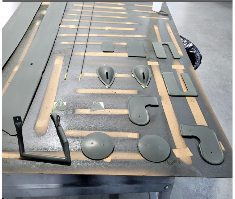
Many small parts have been painted, such as inspection covers, wing fairings, and the step.
