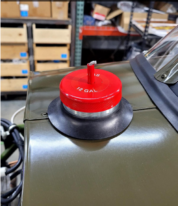
The fuel cap and fuel indicator float are installed.
