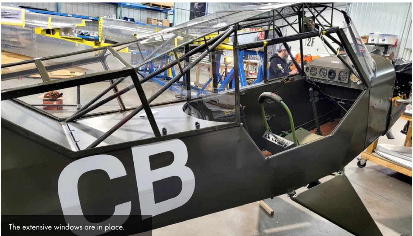
The firewall has been installed.
