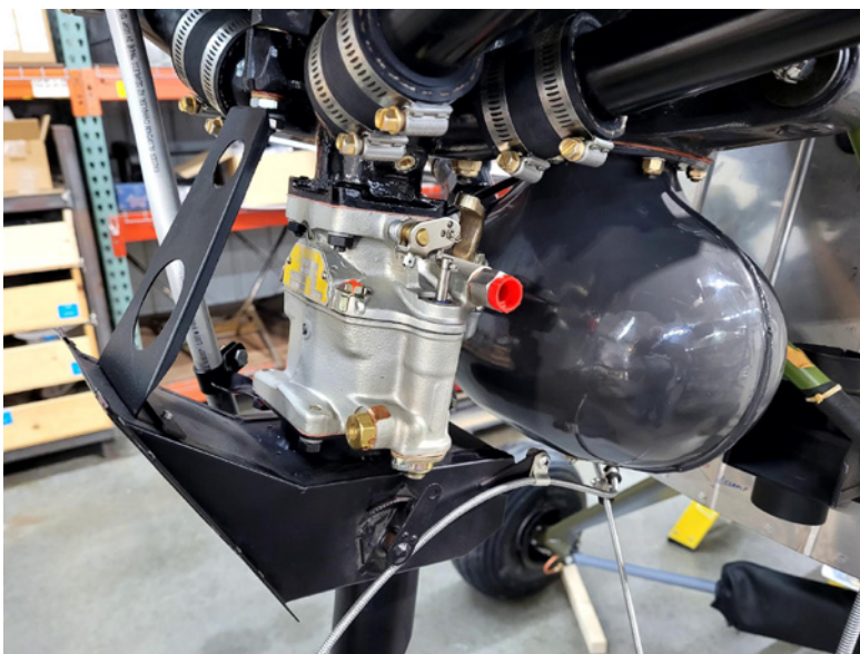
The oil tank, carburetor, and air intake.
