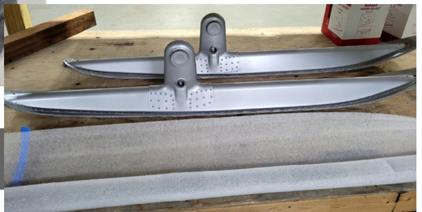
Flying off the snow will be another option for this L-4 when these skis are installed.
