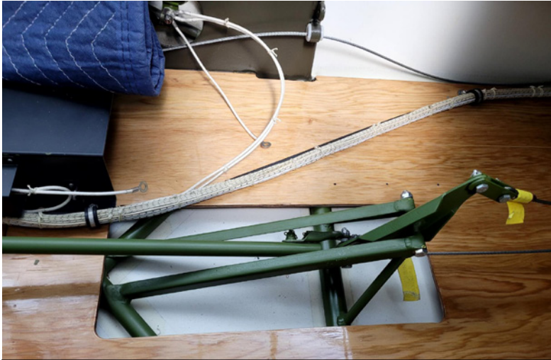
The tubular push rod from the two control sticks connects to a bellcrank that is linked to the elevator by cables.
