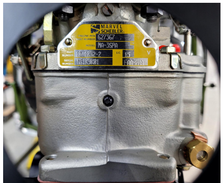
The carburetor is a Marvel Schebler MA-3SPA
