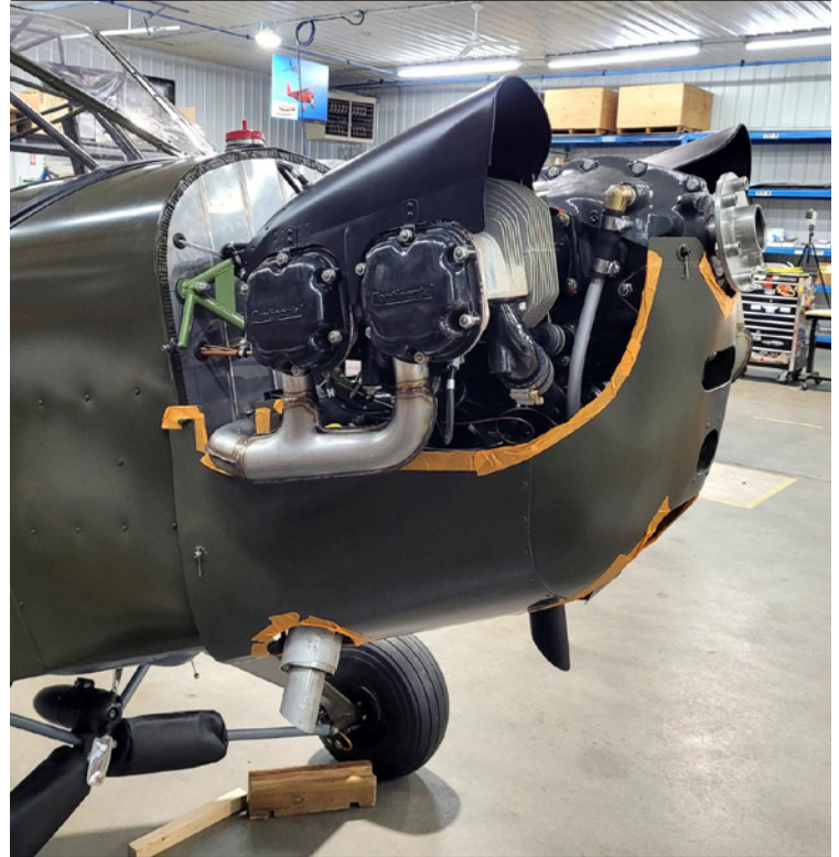
Exhaust and lower cowl are installed.
