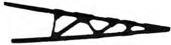
AG-120-TE REPAIR RIB-Lower Trailing Edge
